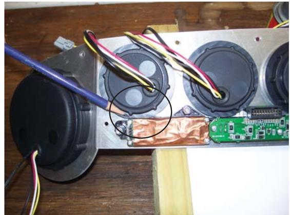
14. The fuel level gauge spacer ring will need to be modified with a dremel tool to give clearance for the odometer display.
