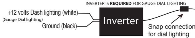
Dial Lighting Inverter Note: Single EL dial lighting inverter included with individual gauge.
